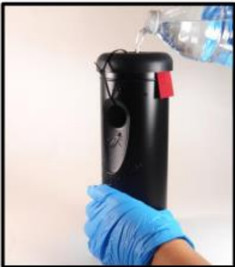
8. Fill trap with water to bottom of drain hole.
